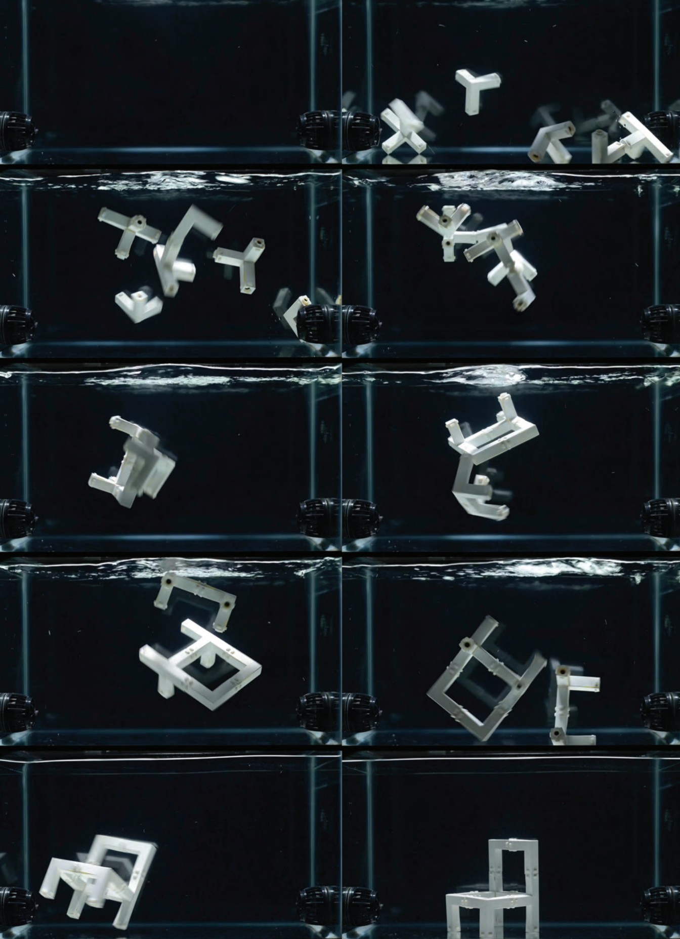
A number of unique components tumble around within a tank of turbulent water, eventually self-assembling into a chair. (Self-Assembly Lab, MIT)
